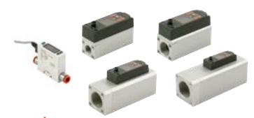
From the communication point of view, a PNP digital output - configurable on the flow rate, pressure or total consumption value - and an analogue output which can be set in voltage (0-10 VDC) or in current (4-20 mA) are available. Versions with IO-Link interface with similar characteristics are also available. The FLUX 1, 2, 3 and 4 can therefore also be used as a flowmeter, flow switch, pressure gauge or pressure switch.
